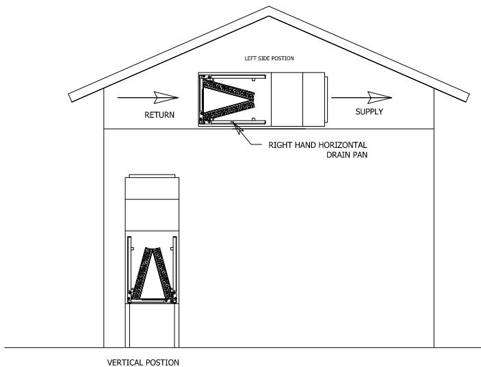
**SL\*/BL\* Multi-Position Air Handlers air flow Up-Flow, Horizontal Left, Horizontal Right.**
